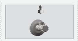
MAKE SURE THAT THE FILTER(S) IS/ARE INSTALLED BETWEEN THE FLEXIBLE PIPE(S) AND THE SHUT OFF VALVE(S) (ANGLE VALVE) (NOT SUPPLIED).
